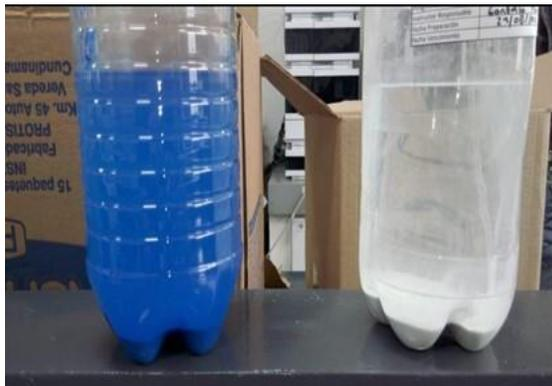
**Figure 6.** Samples after 1 hour of Electrocoagulation
