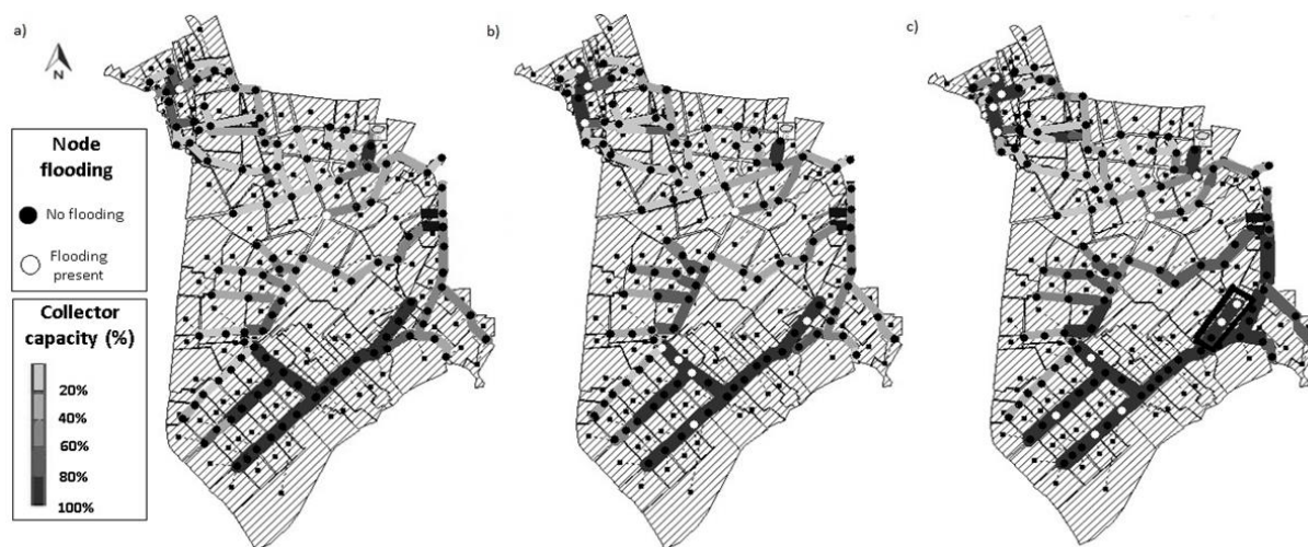
Figure 5. Hydraulic status of the drainage system in the EDZ for a) the current climate scenario, b) the 2030 climate scenario and c) the 2040 climate scenario (own source)
