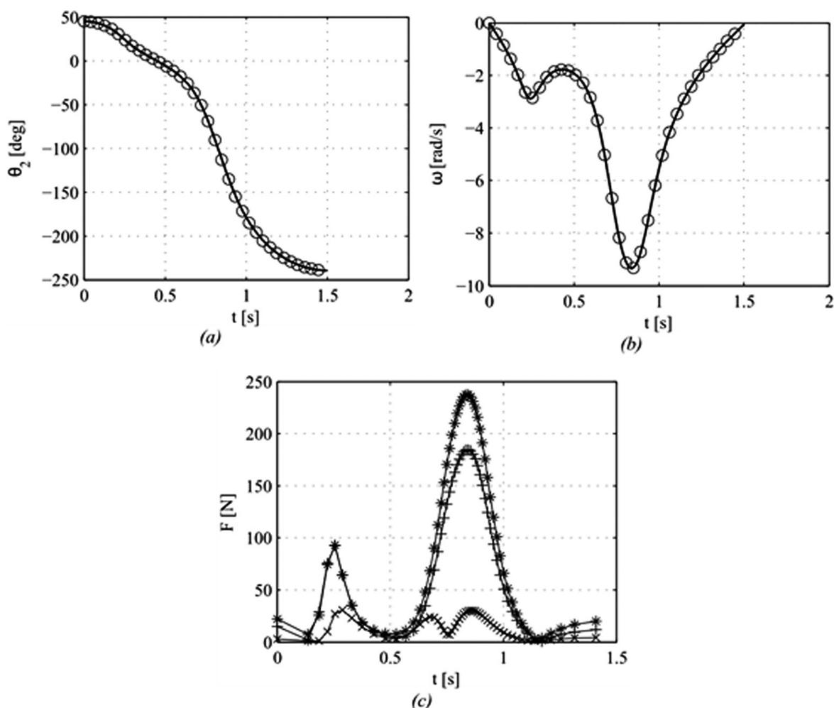
Figure 6. Forward dynamics of the case study's reduced link. a) Generalized coordinate ( $\theta_2$ ). b) Angular velocity ( $\omega$ ). c) Pair reactions ( $F$ ). Convention for the figures a) and b): — modular dynamics; ● commercial MBS. Convention for the figure c): \* reaction in  $O_2$ ; + reaction in A; x reaction in E.
