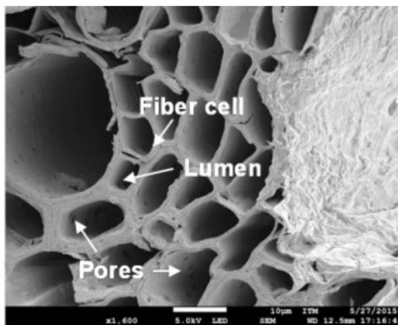
Figure 3. SEM micrographs of untreated pineapple leaf fiber.
