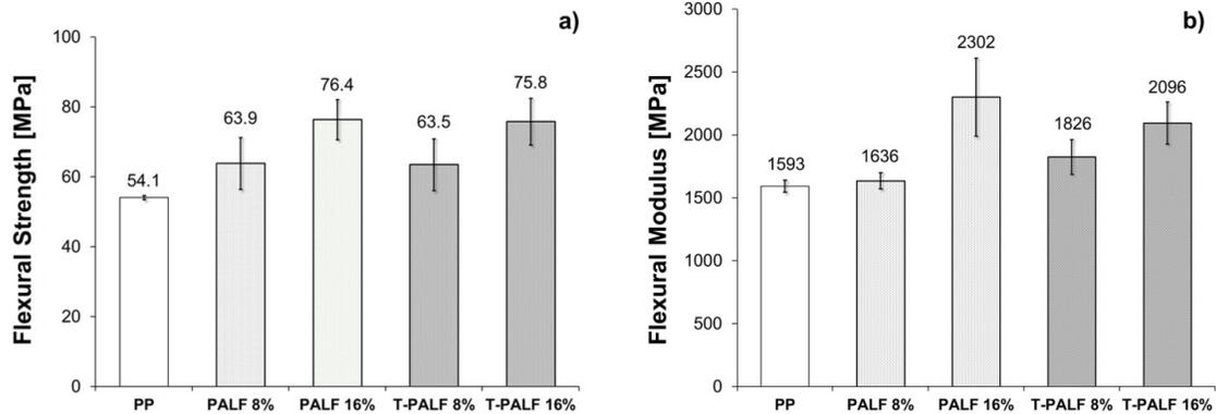
Figure 6. Results from flexural tests of PALF-PP composites. a) Flexural strength b) Flexural modulus. Error bars represent the standard deviation around the expected value.
