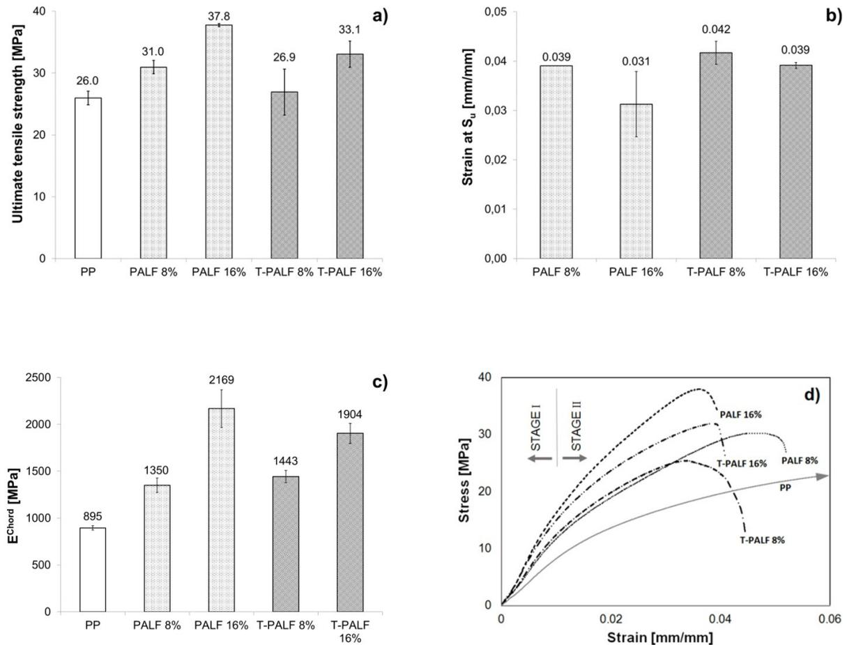
**Figure 4.** Tensile properties of raw fibers (PALF) and treated fibers (T-PALF) polypropylene composites. **a)** Ultimate tensile strength **b)** Strain at ultimate tensile strength ( $S_u$ ), **c)** Tensile chord elastic modulus ( $E_{Chord}$ ), **d)** Tensile Stress-Strain curves of various samples. Error bars represent the standard deviation around the expected value.
