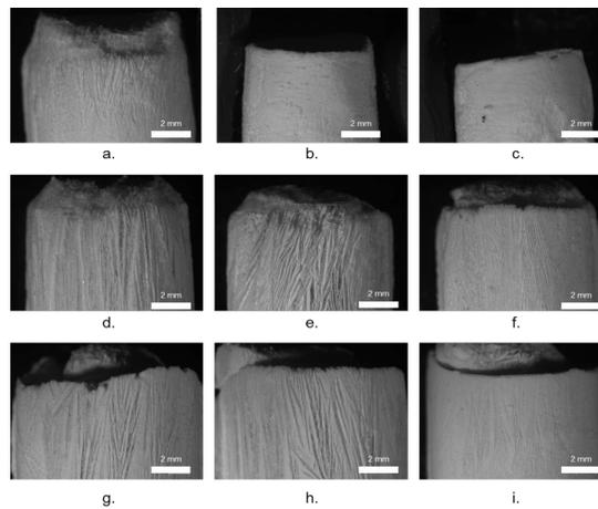
**Figure 4.** Lamellar zone characteristics at different freezing rates and solid content. a. 10% solid content at 0,019 mm/sec. b. 10% solid content at 0,025 mm/sec. c. 10% solid content at 0,081 mm/sec. d. 30% solid content at 0,019 mm/sec. e. 30% solid content at 0,025 mm/sec. f. 30% solid content at 0,081 mm/sec. g. 50% solid content at 0,019 mm/sec. h. 50% solid content at 0,025 mm/sec. i. 50% solid content at 0,081 mm/sec.
