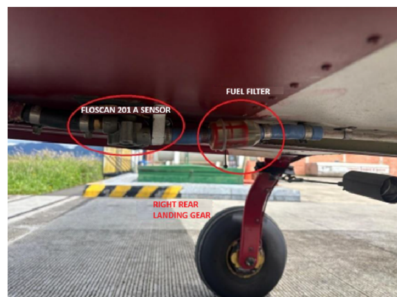
Figure. 6. Installation of the FLOSCAN 201A sensor in the project's LSA aircraft.
