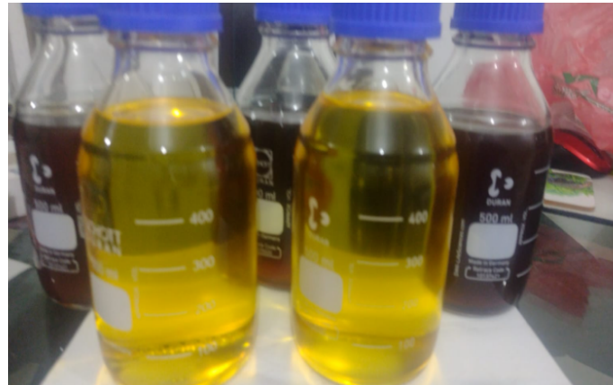
Figure 4. Biodiesel obtained from Sacha Inchi (front) and Sejé (rear) oils
