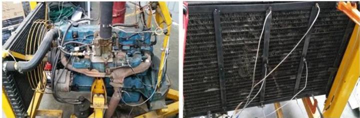
Figure 1. Internal combustion engine (left); radiator on the test bench (right). Source: Own elaboration.
