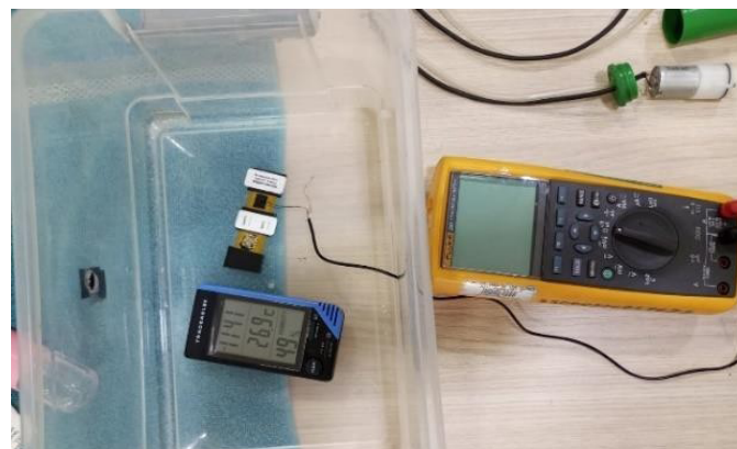
Figure 3. Experimental set-up for humidity test of the sensors
