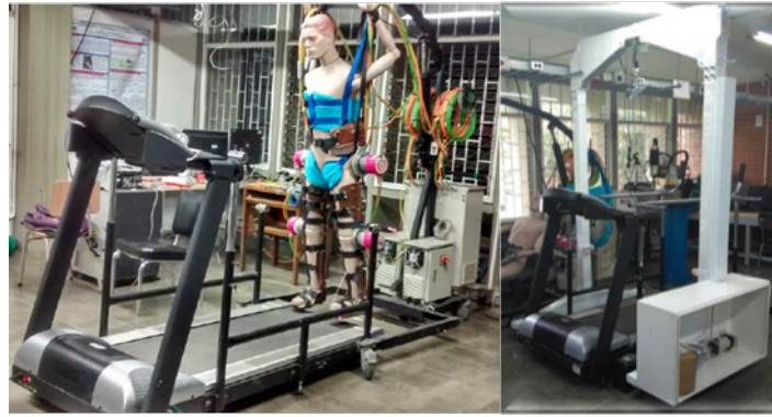
Figure 3. Assisted rehabilitation platform for human gait, RUVEM (14)
