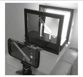
Figure 2. Experimental setup for photoelasticity tests.
