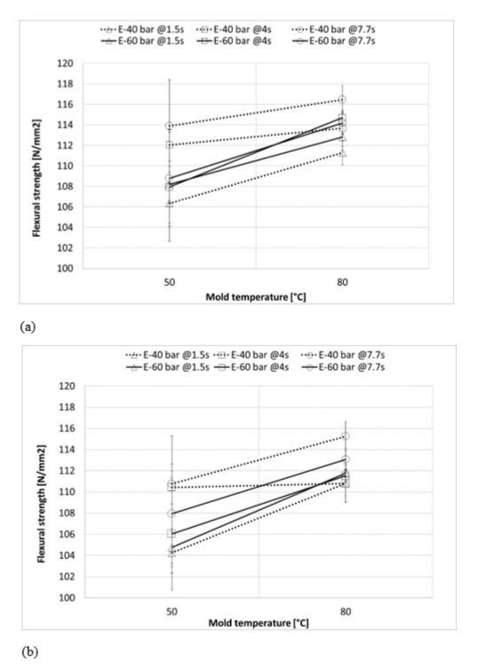
Figure 3. Flexural strength of injected polycarbonate parts with remaining cooling times of (a) 10 seconds and (b) 15 seconds.
