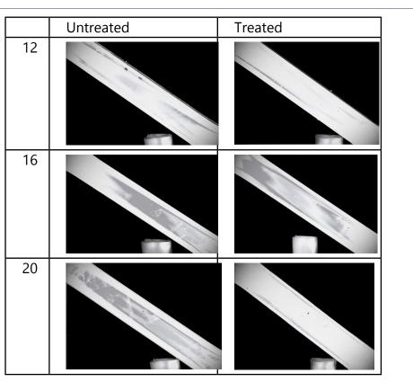
Figure 5. Photoelasticity images of the residual stress patterns in the specimens
