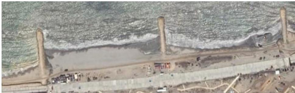
Figure 21. Satellite images. Seawalls 2 and 3. November 2015. [\(33\)](#)
