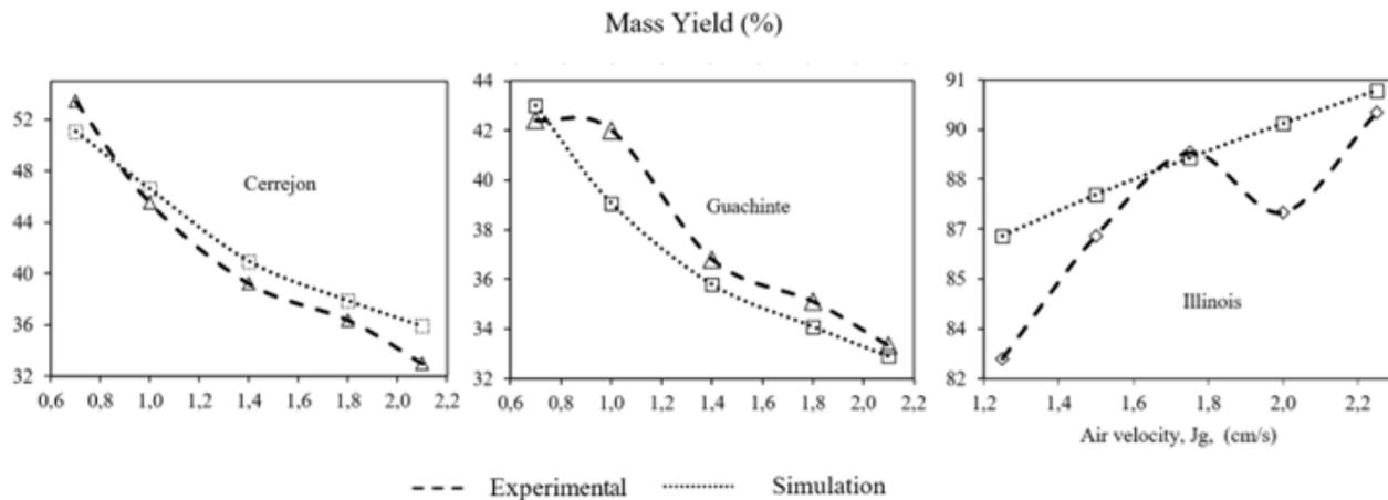
Figure 11. Mass yield vs air velocity ( $J_g$ )
