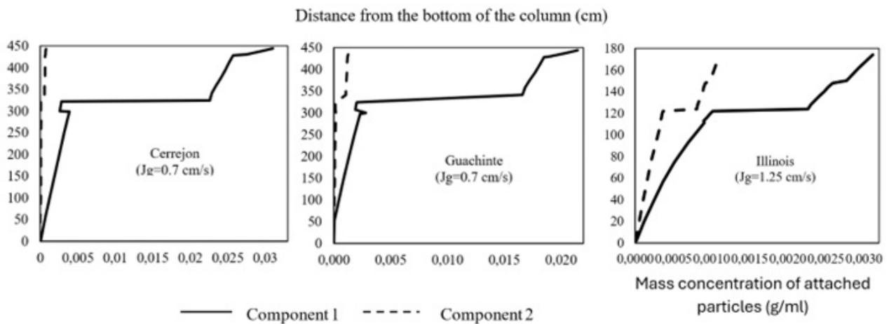
Figure 8. Mass concentrations of attached particles along the flotation column for the organic matter (Component 1) and the mineral matter (Component 2)
