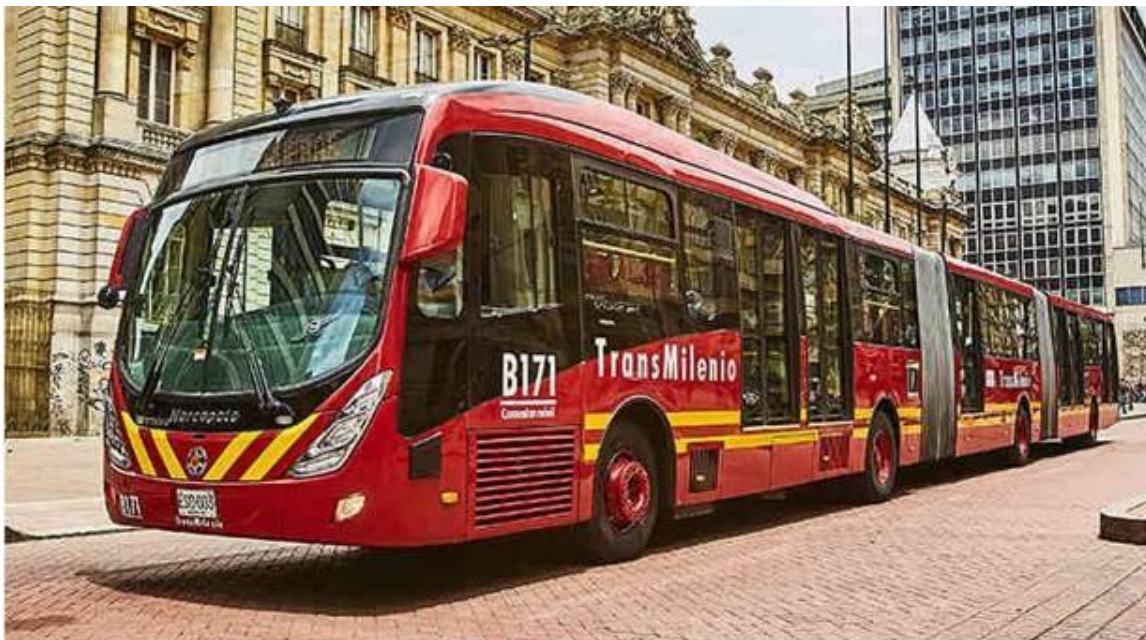
Figure 2. Marcopolo BRT bi-articulated bus on Volvo chassis with central diesel engine. Source: own elaboration
