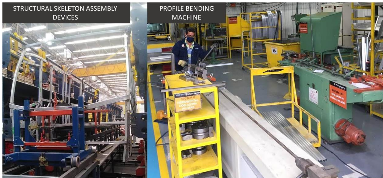
Figure 5. Structural assembly and bending of aluminium profiles with internal development in Superpolo. Source: own elaboration
