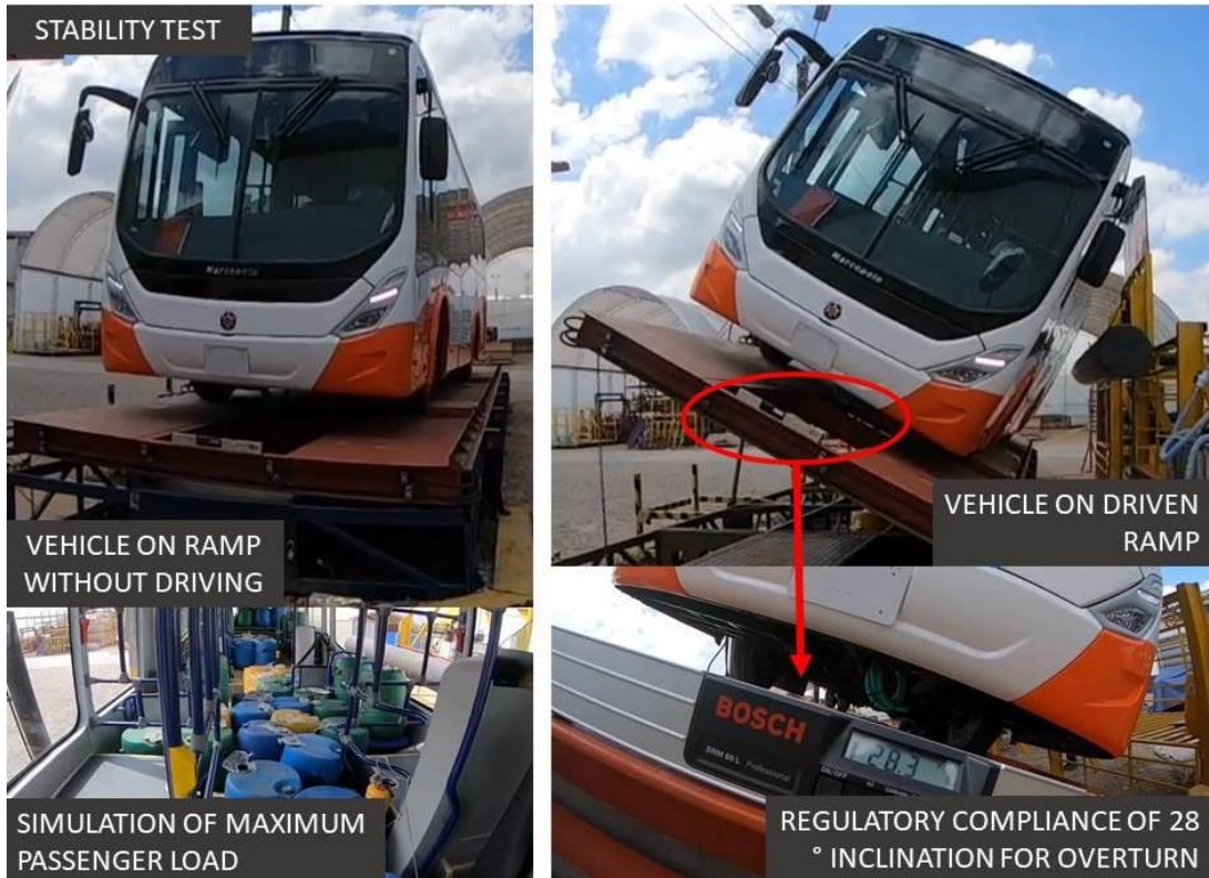
Figure 8. Platform for stability testing. Source: own elaboration
