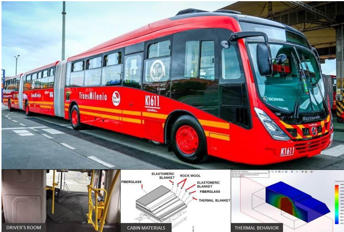
Figure 1. Marcopolo BRT bi-articulated bus on Scania chassis with gas front engine. Source: own elaboration
