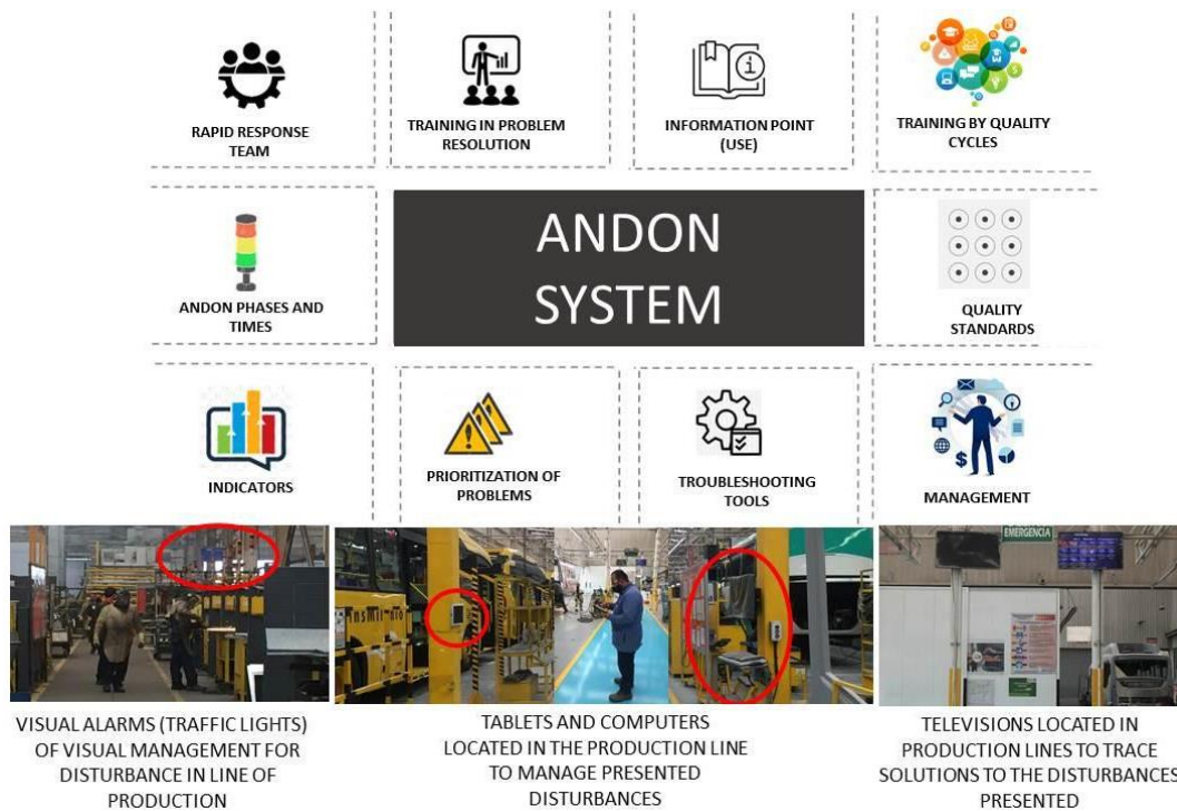
Figure 3. General operating diagram of the Andon system in Superpolo. Source: own elaboration
