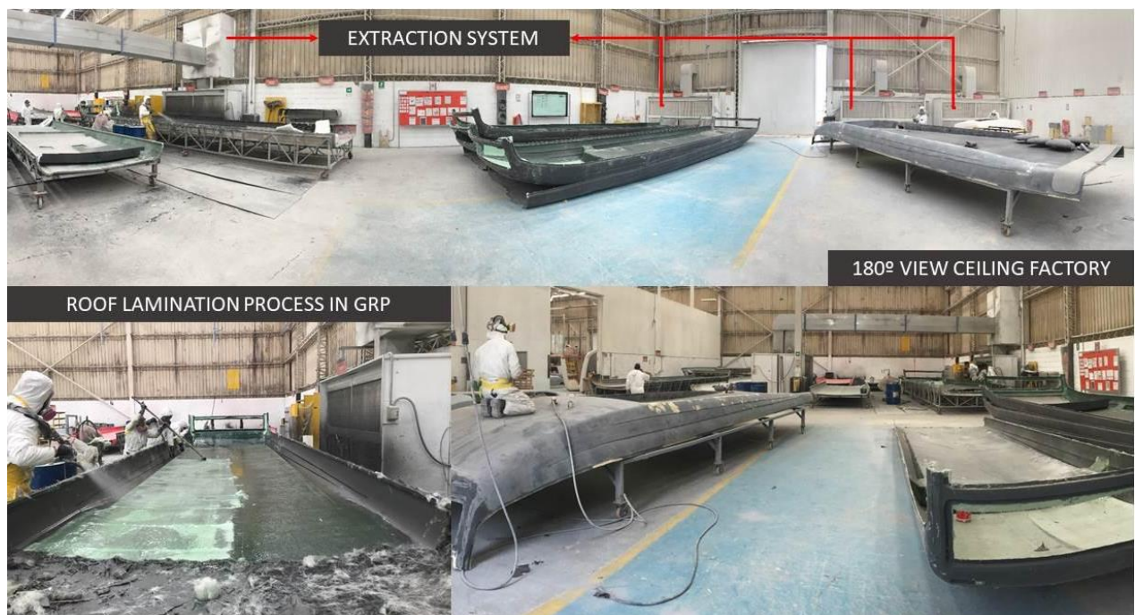
Figure 7. Manufacturing line for GRP roofs. Source: own elaboration
