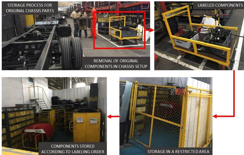
Figure 12. Process of storage and preservation of original chassis components. Source: own elaboration
