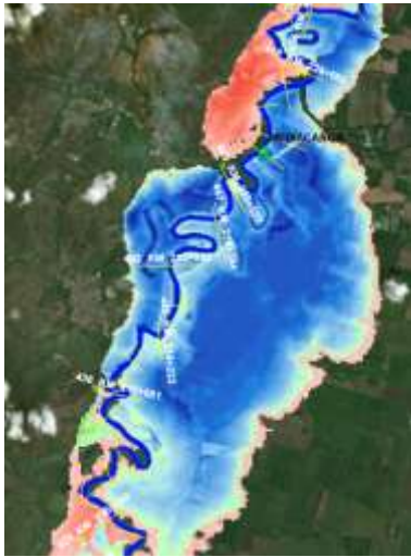
Figure 3. Delimitation of the hydrological component: blue area (flooded area Rt 5), green area (flooded area Rt 15) and red area (flooded area Rt 100)
