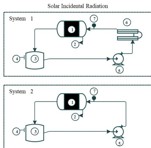
Figure 1. Data Sheet for heat exchanger; reactor systems and study where: 1) CPC reactor; 2) involute; 3) tank, 4) sampling; 5) recirculating pump; 6) heat exchanger; and 7) thermocouple viewfinder.
