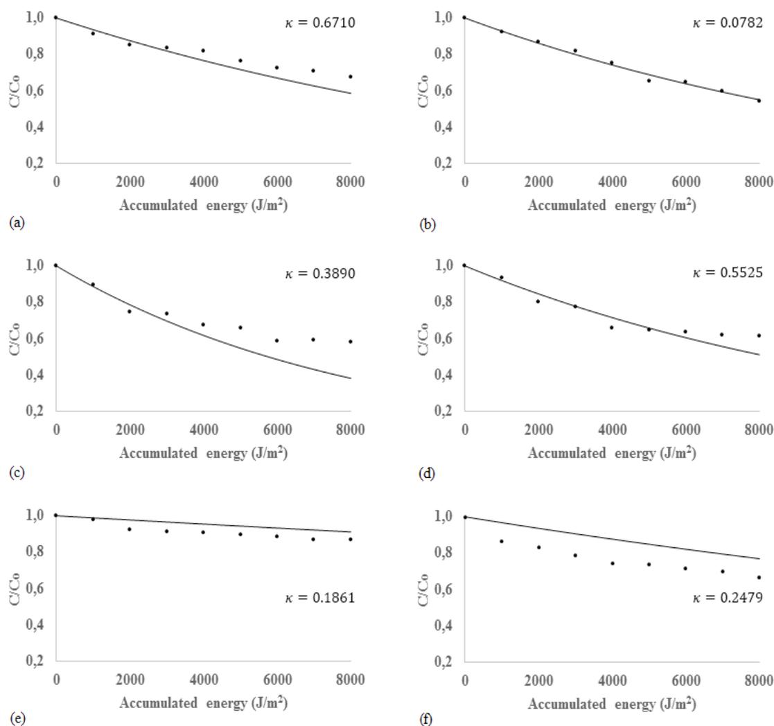
**Figure 5.** Adjusting experimental kinetic data for the solar heterogeneous photocatalytic degradation CPC reactor: (a) not preheated to 306 K, (b) not preheated to 305 K, (c) preheated to 323 K, (d) preheated to 321 K, (e) isothermal at 307 K and (f) at isothermal at 318 K.. Experimental data (●), Reaction rate model (-). The model reaction rate includes the effect of temperature.
