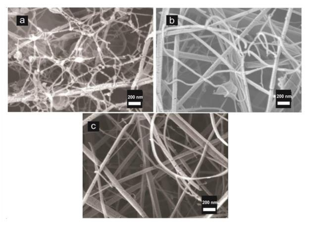
Figure 3. SEM micrographs of QS:FGS scaffolds to 50000x different weight ratios (a) QS/FGS (3: 1), (b) QS:FGS (1: 1) and (c) QS:FGS (1:3). taken at IIM-UNAM.
